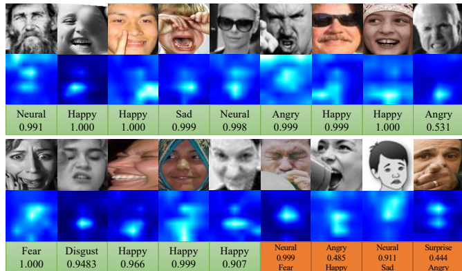
Fig. 4. An illustration of the learned attention maps. The first row is to show the raw images, the second row is the attention maps of the MTE, and the corresponding predictions or the labels are shown in the third row. The annotations marked in green are the predicted expressions and their confidence scores, while the others in orange are false predictions with the ground-truth labels annotated.
